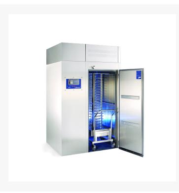
Williams Roll In WMBC320C 1 Door Combi Blast Chiller Cabinet has 320 kg of storage capacity, 1670mm (W) x 2350mm (D) x 2295mm (H) dimension size, 650kg of weight, 1 solid door, stainless steel finish, accommodates 1/1 or 2/1 Gn combi mobile rack, and R404a refrigerant gas.
